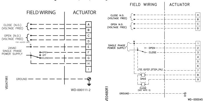
Figure 2. 24 Vac Wiring 5000 lb.-in. Models.
