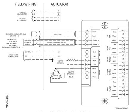
Figure 5. 120 Vac Modulating.
