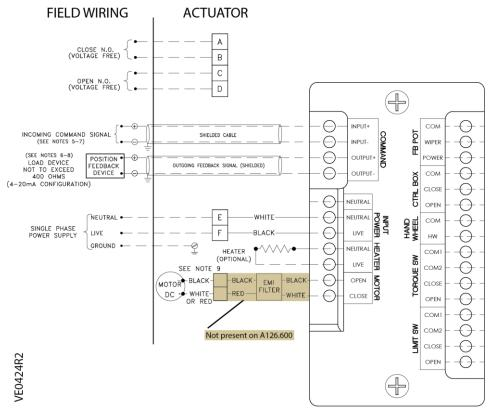
Figure 4. 24 Vac Modulating.
